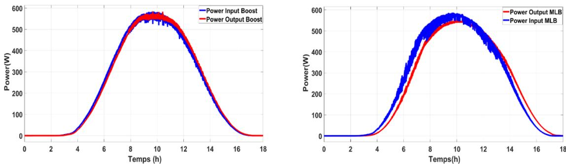
Fig 9. Output power (a) Traditional boost converter (b) Multi-Level boost converter
