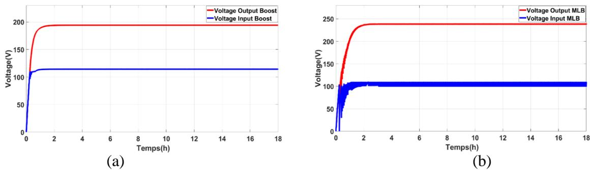
Fig 4. Output voltage (a) Traditional boost converter (b) Multi-Level boost converter
