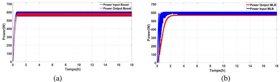
Fig 5. Output power (a) Traditional boost converter (b) Multi-Level boost converter
