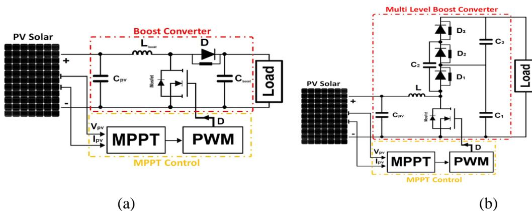
Fig 2. DC/DC converters for PV stand-alone application (a) Traditional boost converter (b) Multilevel boost converter (MLBC) [3]
