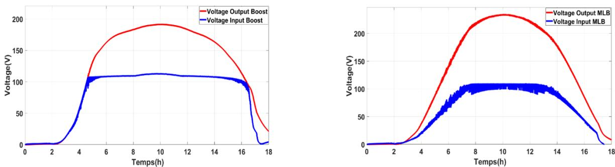
Fig 8. Output voltage (a) Traditional boost converter (b) Multi-Level boost converter
