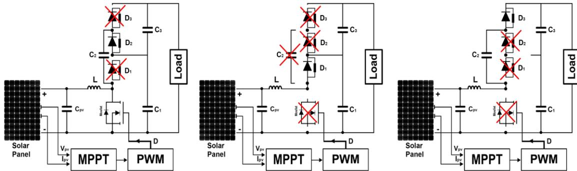
Fig 3. Multi-level Boost Converter (a) Switch is ON (b) Switch is OFF ( $D_1$ ) (c) Switch is OFF ( $C_2, D_3$ ) [9]
