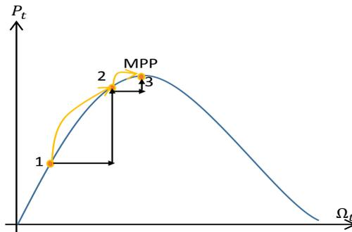
Fig 3. Maximum power searching using fuzzy MPPT technique
