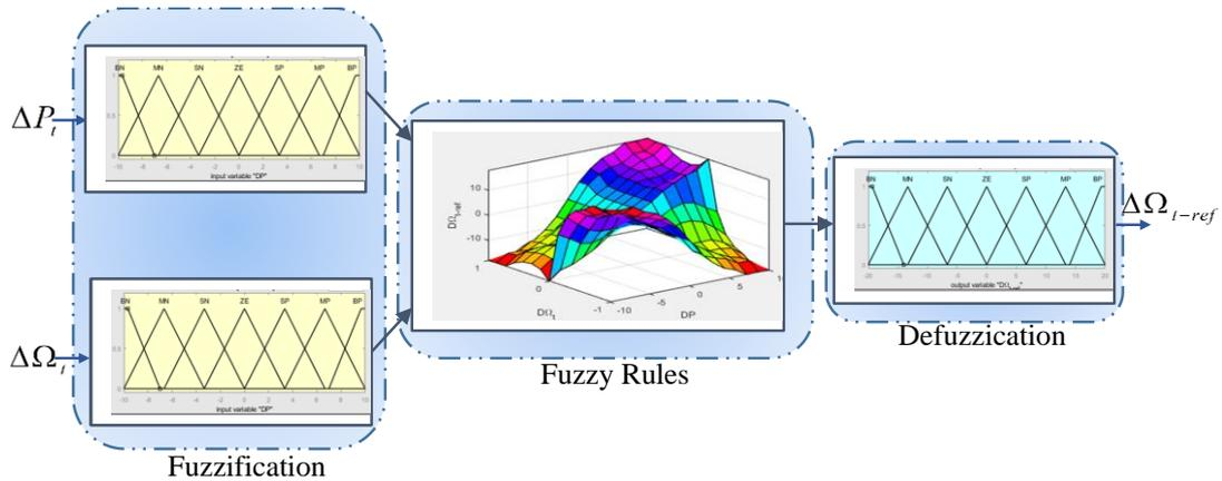
Fig 4. Fuzzy logic controller bloc
