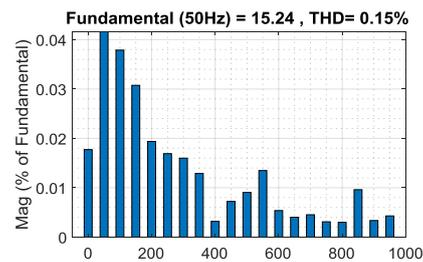
Fig 11. Harmonic spectrum of the stator current obtained with 3LVSI-DTC
