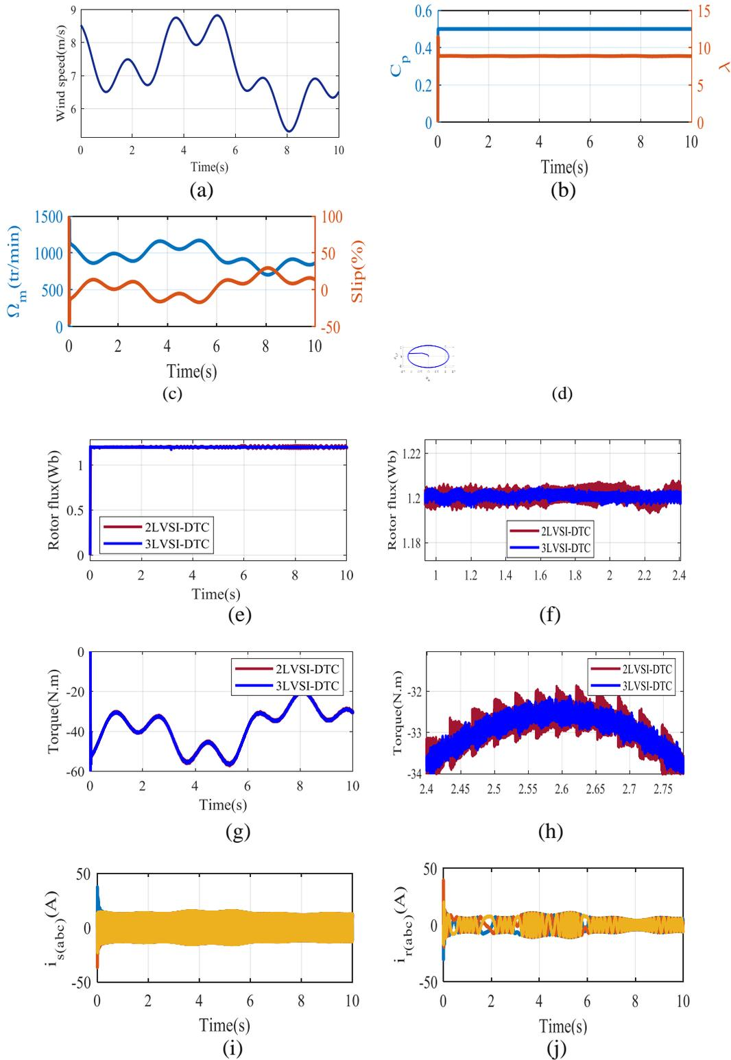
Fig 9. Simulation results of the proposed control, (a) Wind speed profil, Rotor flux, (b) Aerodynamic efficiency and speed ratio, (c) Rotational speed and slip,(d)(e) Rotor flux, (f) zoom of rotor flux, (g) Torque, (h) zoom of torque, (i) Stator current waveform, (j) rotor current waveform.
