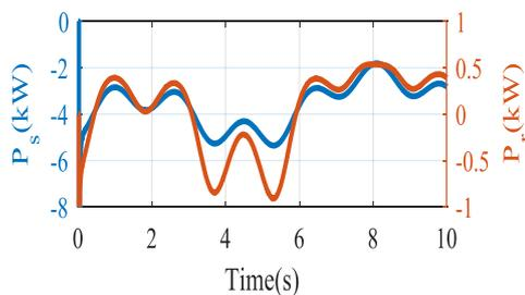
Fig 10. Waveforms of the stator and rotor active power.
