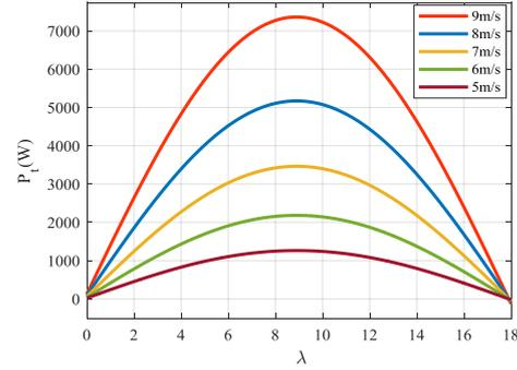
Fig 2.  $P_t(\lambda)$  for different wind speeds
