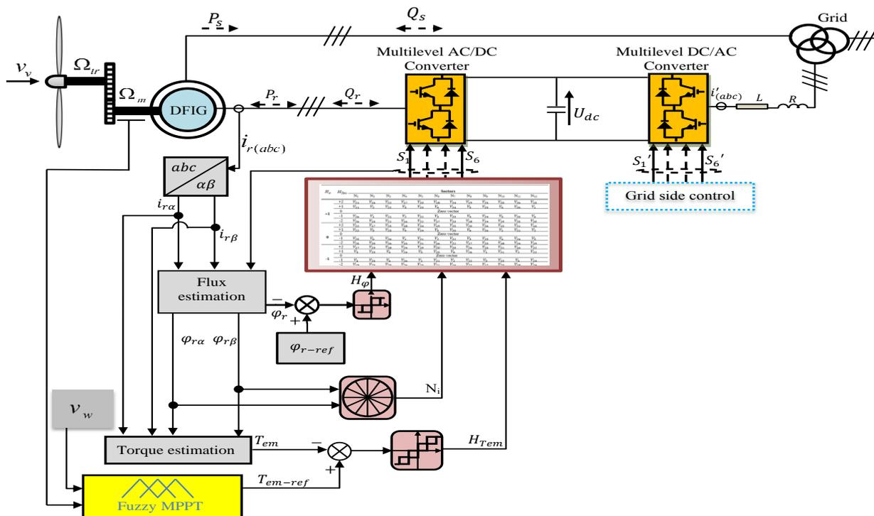
Fig 8. Block diagram of WT-DFIG control by 3L VSI-DTC based on fuzzy MPPT.
