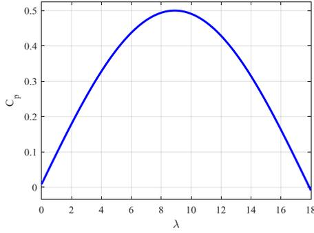
Fig 1.  $C_p(\lambda, \beta)$  Characteristic for  $\beta = 0^\circ$
