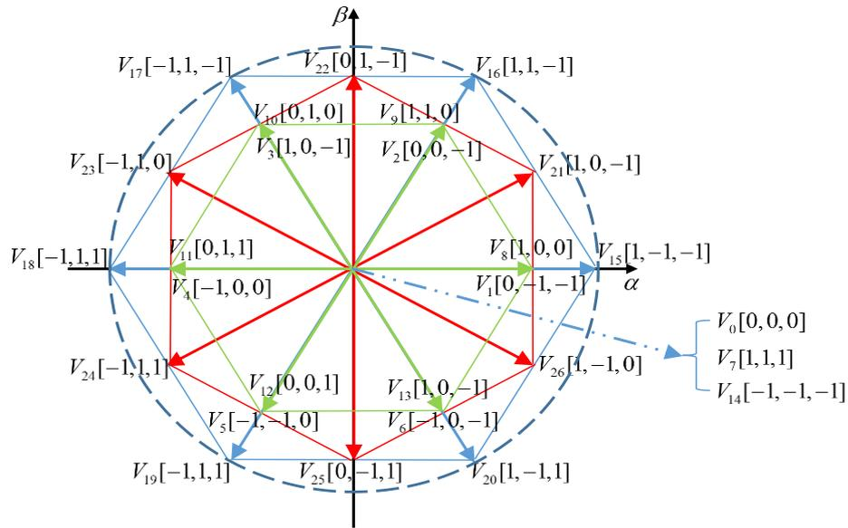
Fig 7. Voltage vectors provided by the three-level inverter
