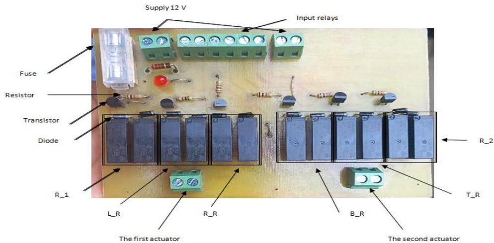
Fig. 6 Relays circuit.
