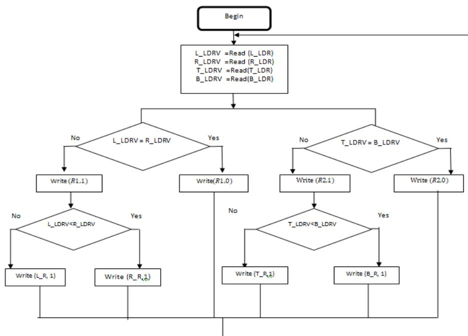
Fig. 5 Flowchart of C programming code implemented in Arduino Uno Board.
