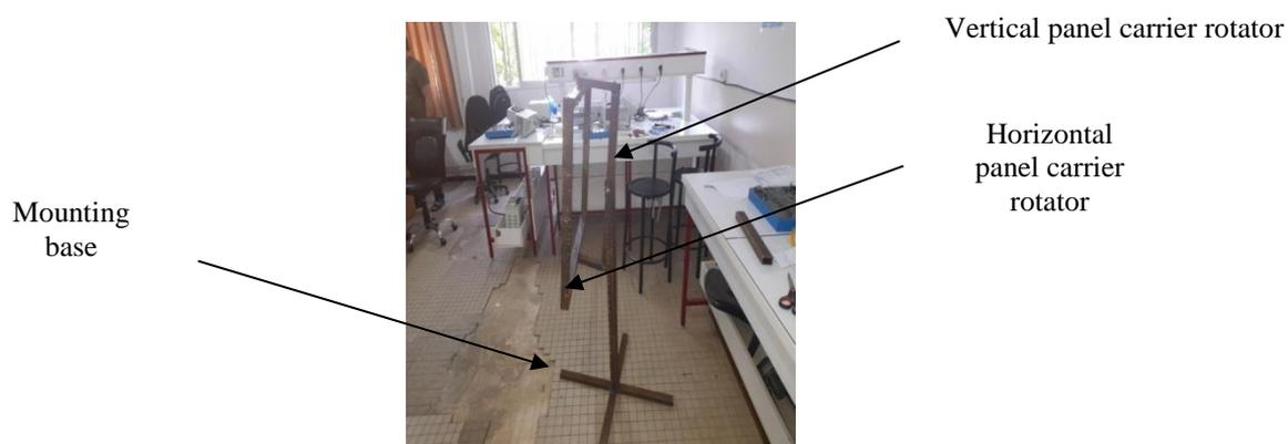
Fig. 1 The mechanical part.
