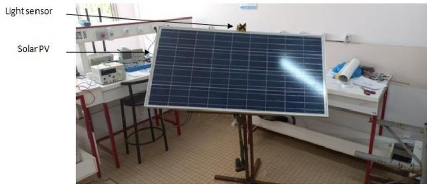
Fig. 7 Proposed dual axis solar tracker system.
