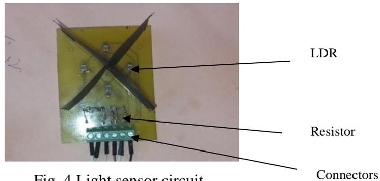
Fig. 4 Light sensor circuit.
