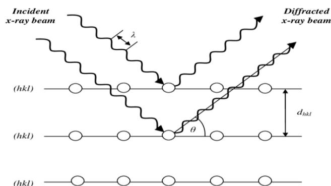
Fig. 6. Diffraction of incident X-ray beams on the crystallographic planes[24].
