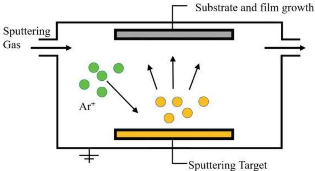
Fig. 5. Conventional diagram of a sputtering system [23].
