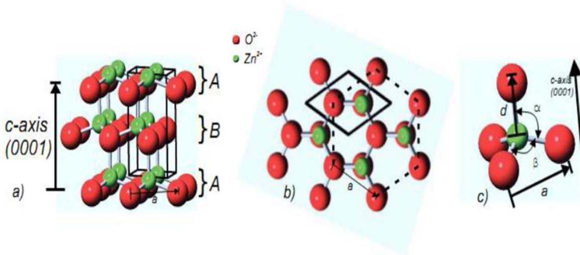
Fig. 4. Compact hexagonal structure of Würtzite.
