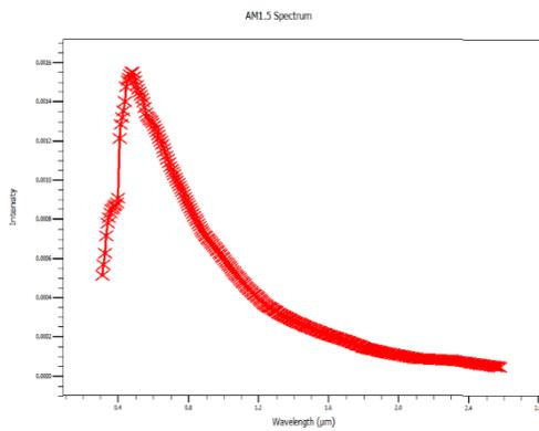
Figure 2. The solar spectrum used AM1.5
