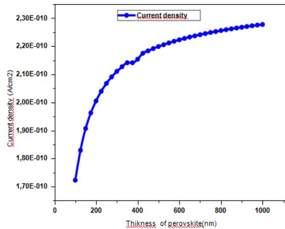
Figure 9. Jsc as a function of region 2 thickness
