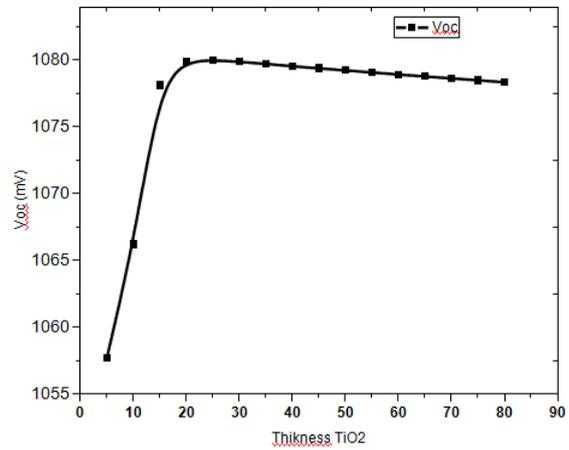
Figure 7. Voc as a function of region thickness 1
