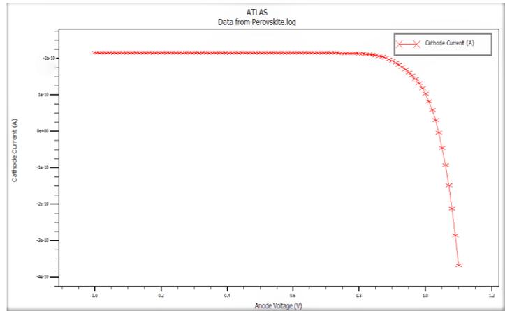
Figure 3. I-V characteristic of the reference perovskite-based solar cell
