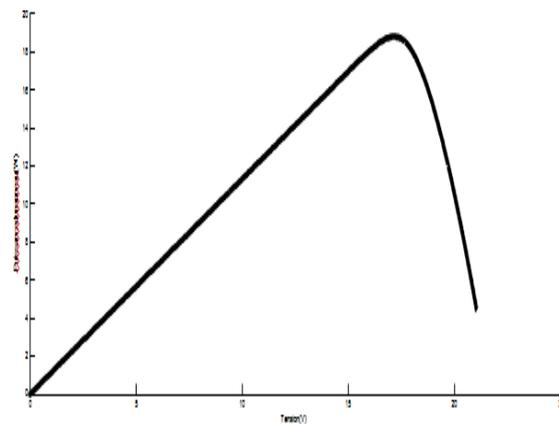
Figure 16. P-V characteristic of the perovskite-based solar panel
