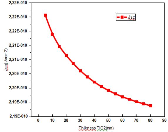
Figure 5. Jsc as a function of region 1 thickness
