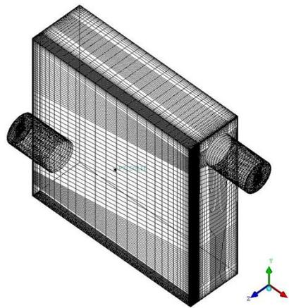
Fig 2 Fluid and solid merged meshes
