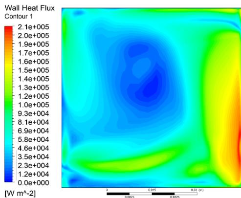
Fig 5. Wall heat flux at the fluid-solid interface
