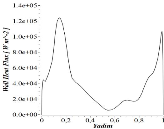
Fig 9. Wall heat flux at the perpendicular middle line of the fluid-solid interface
