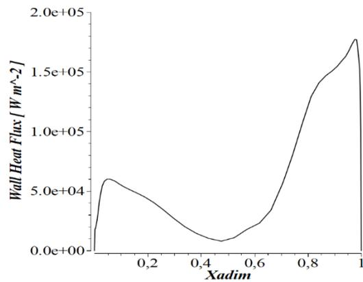
Fig 10. Wall heat flux at the horizontal middle line of the fluid-solid interface
