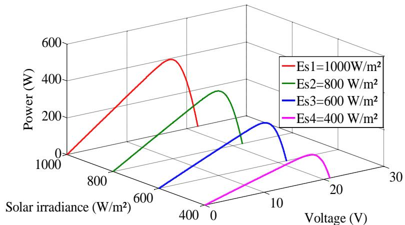
Fig 3. PV electrical characteristics
