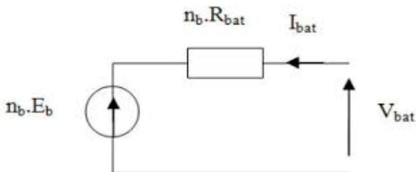
Fig. 4 Battery electrical model
