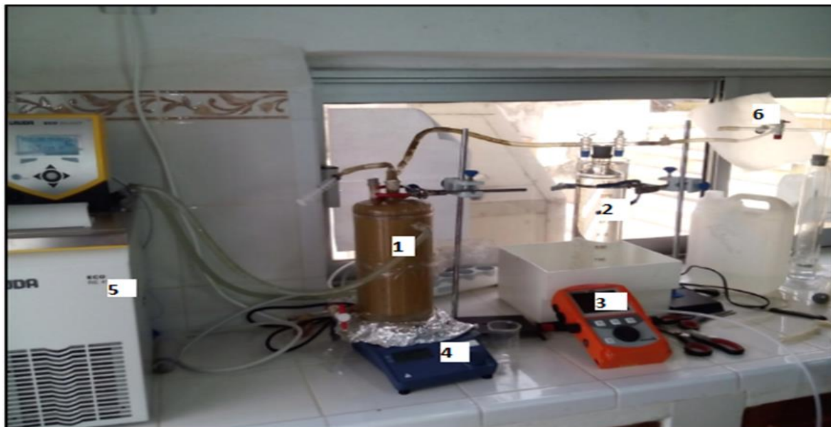
Fig. 1. Photographic view of the digester (1): Double wall reactor 1.5 L ;(2) Glass gasmeter; (3): Portable biogas analyzer; (4): Stirring plate; (5): Thermostat bath with a Temperature set at 55°C; (6): Tedlar bag.
