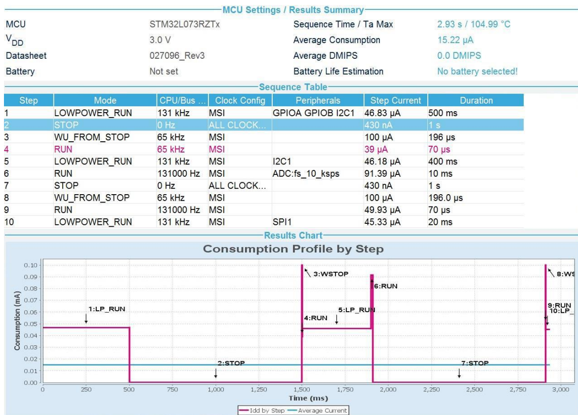
Fig 4. Energy consumption estimation for the STM32L073RZ
