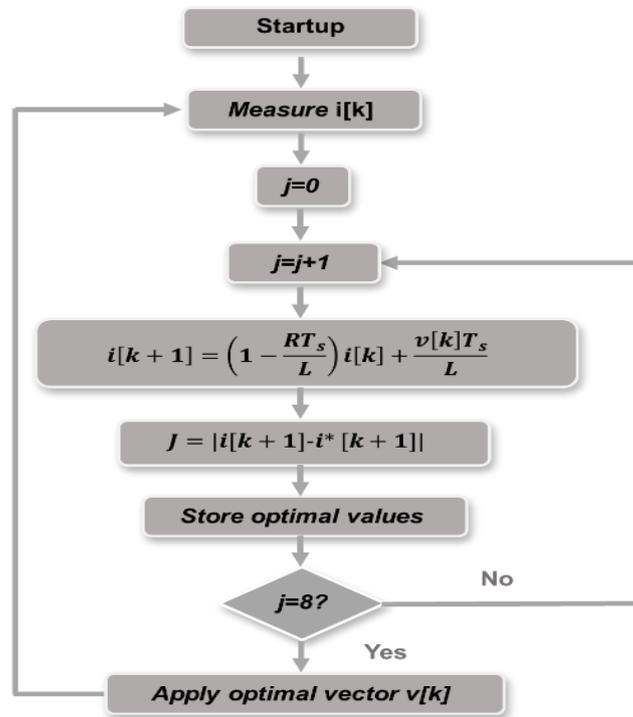
Fig 4. Flow diagram of MPCC.
