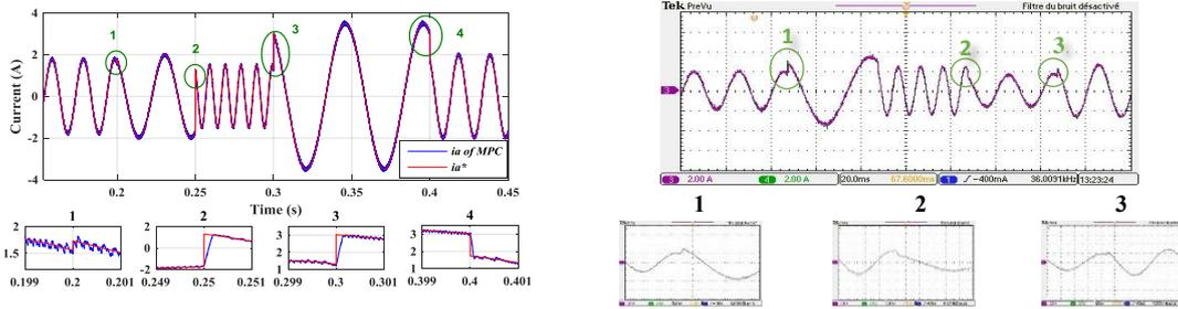
Fig 8. Simulation and experimental results of: reference and output current of phase (a) and their zoom.
