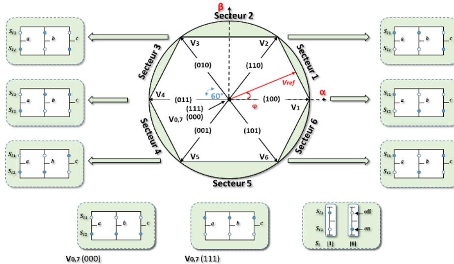
Fig 5. Eight possible combinations of the switching signals, and their corresponding voltage vectors generated by the inverter in the complex plane
