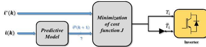
Fig 3. Predictive current control block diagram
