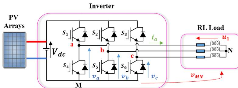
Fig 2. Voltage source inverter power circuit
