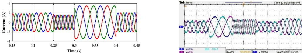
Fig 7. Simulation and experimental results of: output current of three phase.
