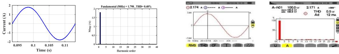
Fig 9. Simulation and experimental results of: output current of phase (a) and their THD.
