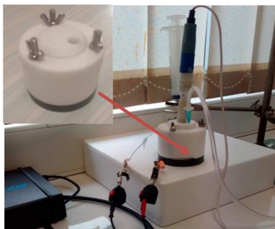
Fig. 1. The electrolysis cell under controlled atmosphere, N 2 gas.
