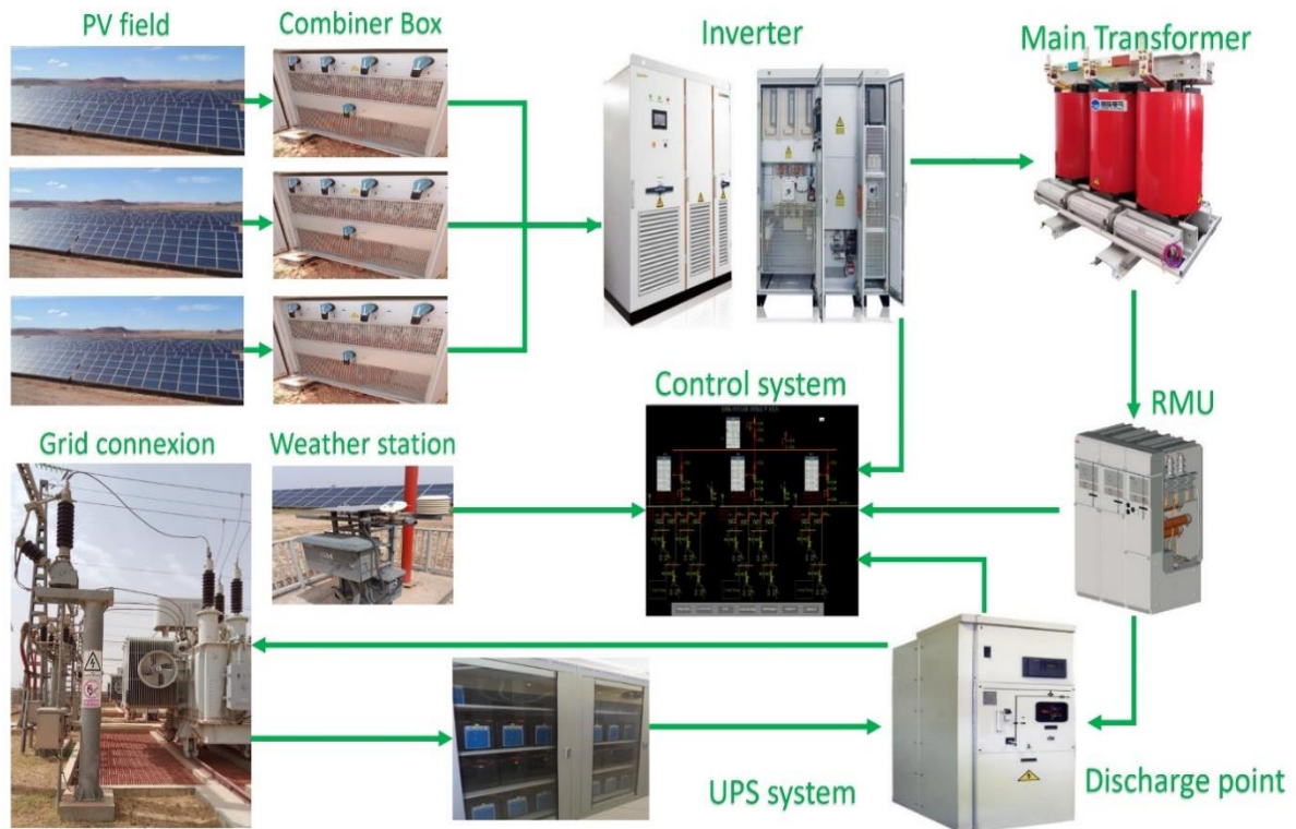
Fig 5. Schematic diagram of the 53MW Djelfa solar power plan
