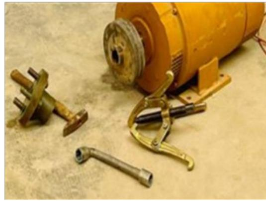
Fig 7. Installation of the pulley on the generator
