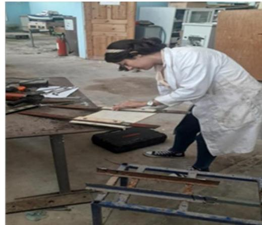
Fig 8. Drilling of Flat Irons and Assembly of the Jig System
