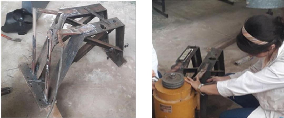
Fig 9. Welding of flat irons using the jig and Mounting of the generator with the bracket
