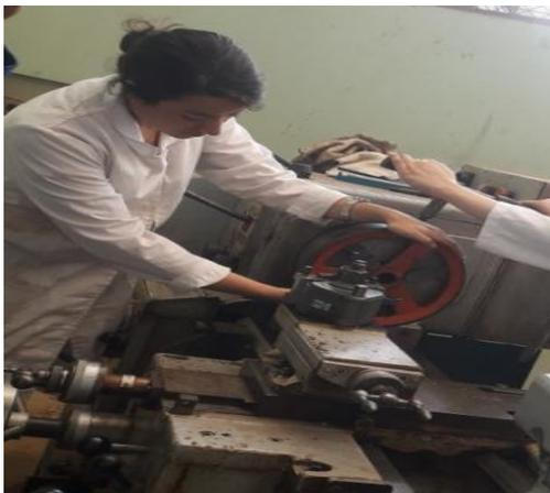
Fig 4. Lathe machining of pulley center section
