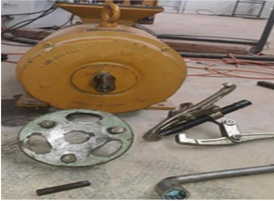
Fig 6. Generator pulley extraction
