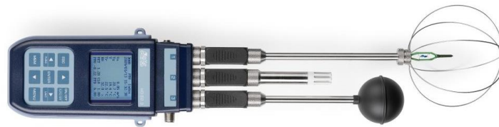
Fig 4. HD32.2 WBGT Index instrument (Delta OHM, Italy)
