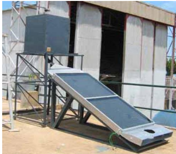
Fig 1. Natural convection solar dryer at CDER (Boulemtafes-Boukadoum et al., 2008)
