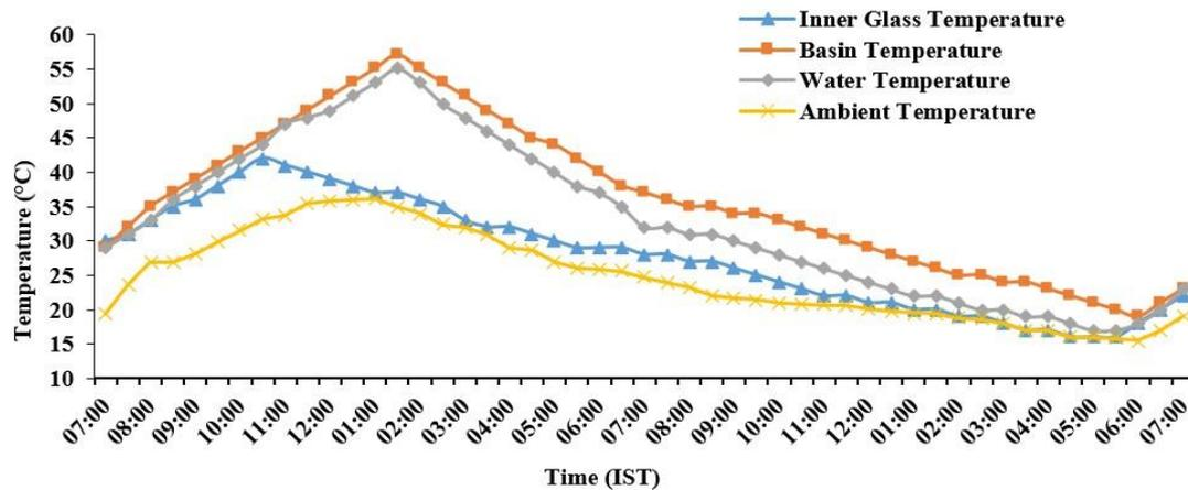
Fig. 4. Variation of various temperatures with time for CSS without PCM.
