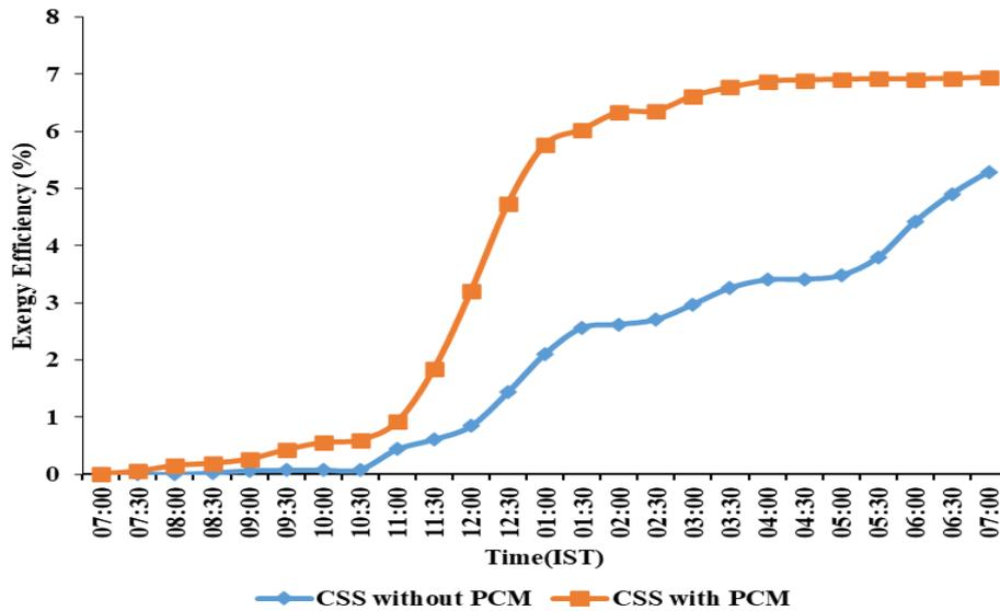
Fig 7. Variation of exergy efficiency with time for CSS without PCM and CSS with PCM.
