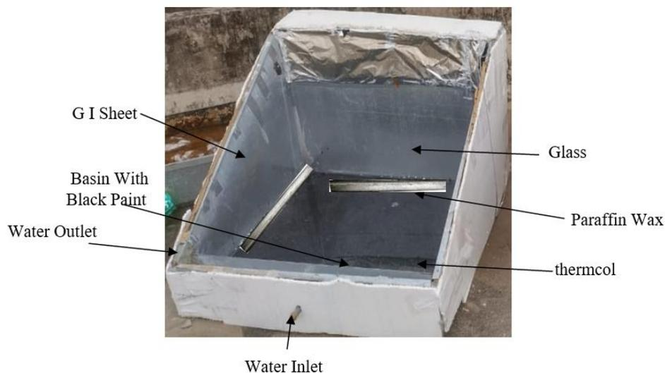
Fig 1. Schematic picture of the experimental setup illustrating various parts.
