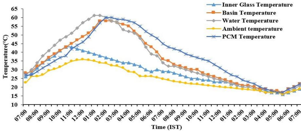
Fig 5. Variation of various temperatures with time for CSS with PCM.
