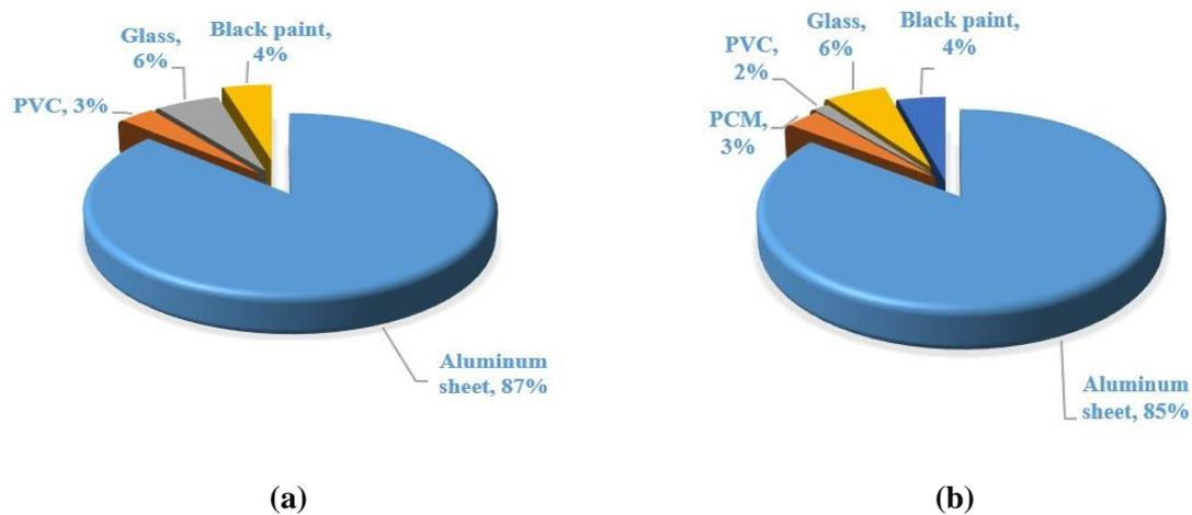
Fig 9. Distribution of embodied energy for different components used in CSS (a) without PCM, (b) with PCM
