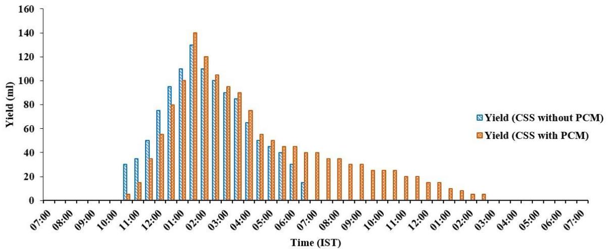
Fig 8. Variation of yield of water with time for setups CSS without PCM and CSS with PCM
