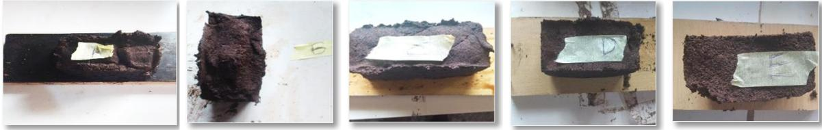
Fig 1. PKS Briquette Samples Produced for Assessment
