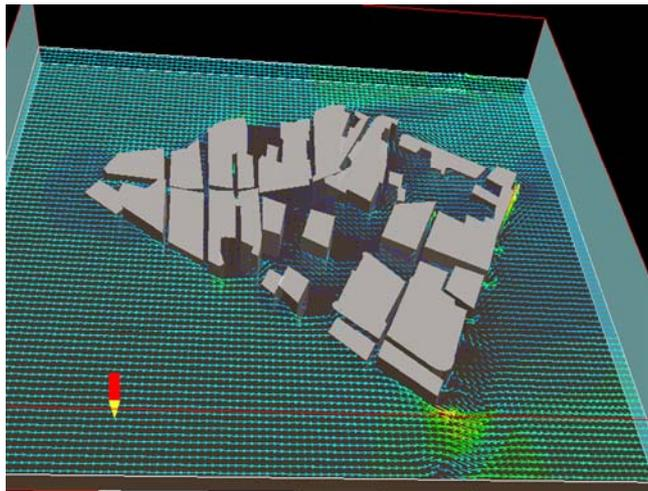
Fig. 8: 3D view of the horizontal distribution of airflow at the height of 8 m in the sample area
