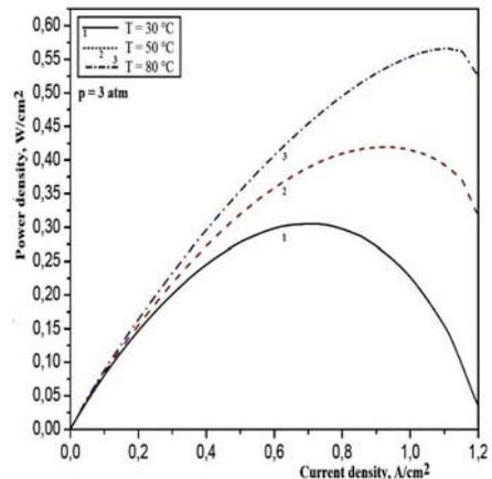
Fig. 5: Power density vs temperature
