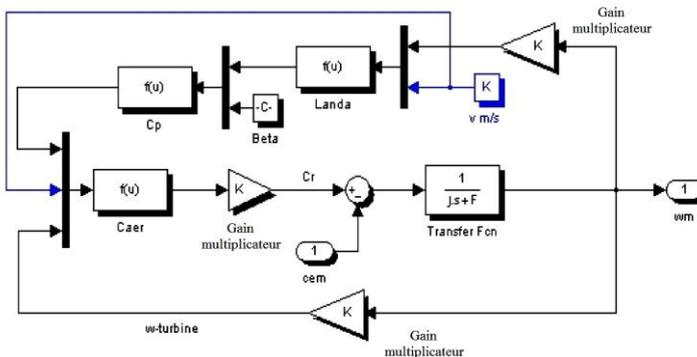
Fig. 9: Model of the turbine
