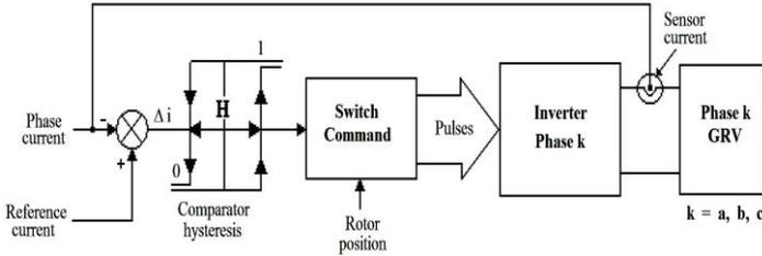
Fig. 5: synoptic diagram of the proposed single phase control circuit
