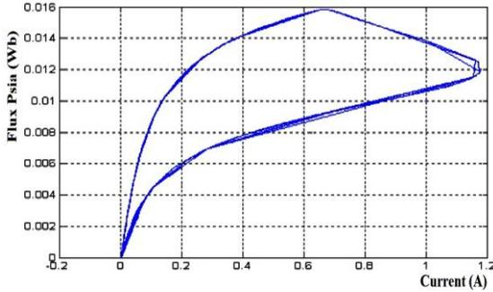
Fig. 15: Energy conversion cycles for the SRG of Fig. 1(speed=5000 rpm)
