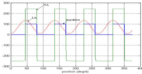
Fig. 16: Influence of the pulses on the voltage and the inductance of the machine
