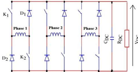
Fig. 4: Power Inverter system of three-phase SRG
