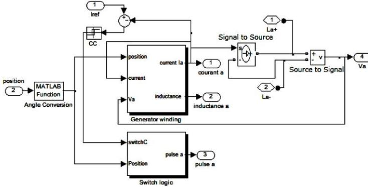
Fig. 6: The simulation model of phase (a)
