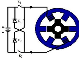
Fig. 1: SRG diagram and associated converter
