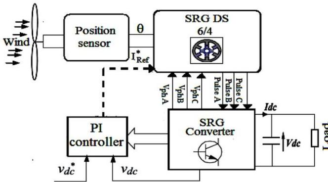
Fig. 11: Simulation model of SRG system
