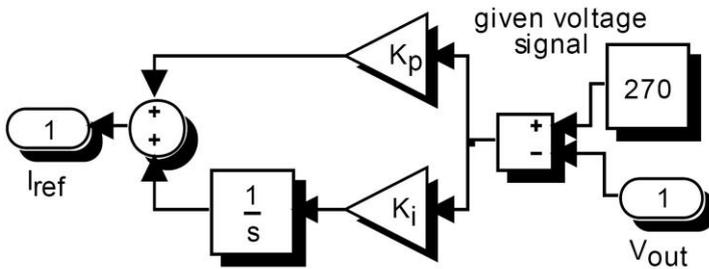
Fig. 8: Simulation model of outer voltage controller
