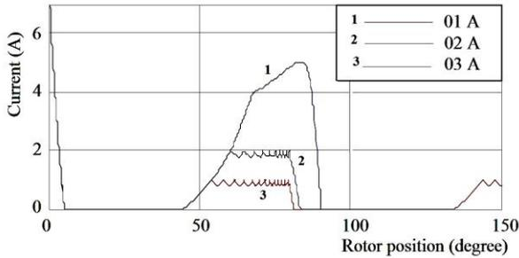
Fig. 13: Simulation waveforms of phase current with CCC ( $\theta_{on}=45^\circ$ ,  $\theta_{off}=80^\circ$ , speed=3000 rpm).
