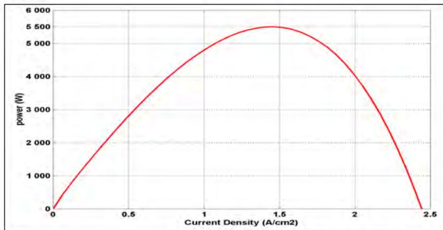
Fig. 4 5.5kW PEMFC P-I Characteristic.
