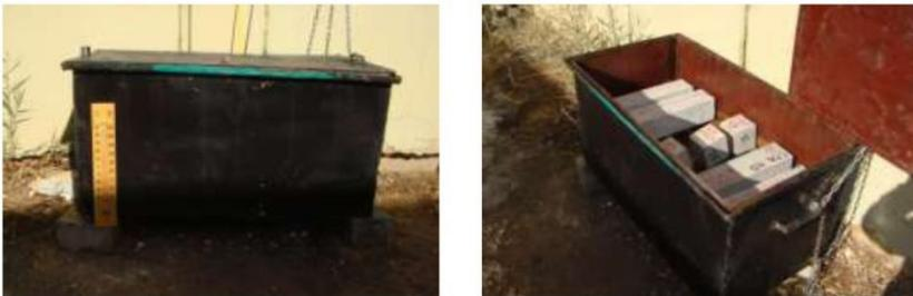
Fig. 2: Steam curing chamber exposed to solar radiation
