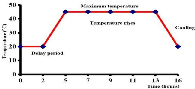
Fig. 4: Schematic representation of steam curing (1 cycle)
