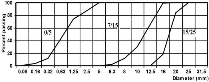
Fig. 1: Grading curves of sand and gravels
