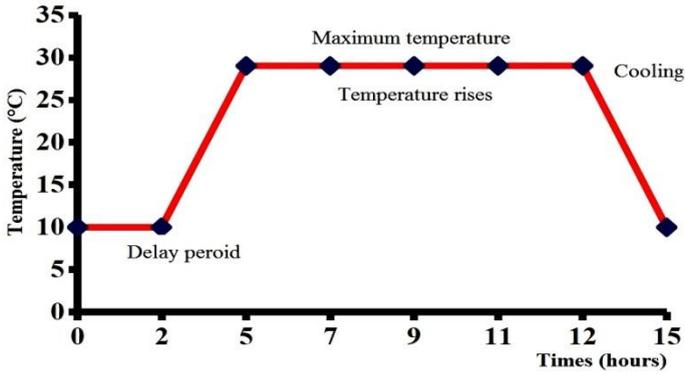
Fig. 5: Schematic representation of steam curing (2 cycle)
