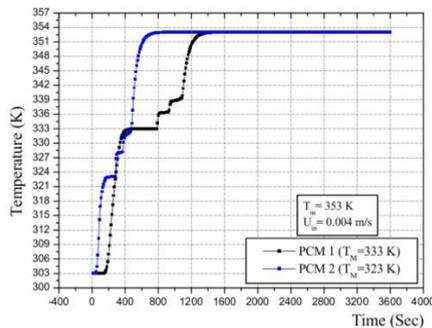
Fig. 2c: Unsteady temperature evolutions of PCM1 and PCM2 ( $T_{f,in} = 353$  K)
