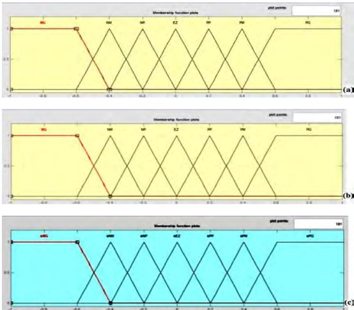
Fig. 10: Membership function for error and control of speed and hysteresis flou controller
