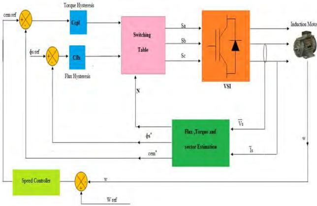
Fig. 3: Block diagram of DTC
