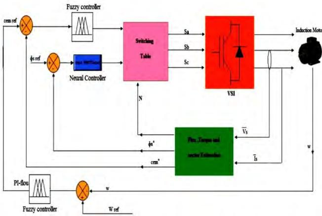
Fig. 5: Three-level DTC with 24 sectors based on artificial intelligence techniques of an induction machine
