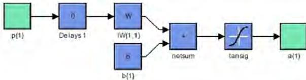
Fig. 7: Structure of layer 1
