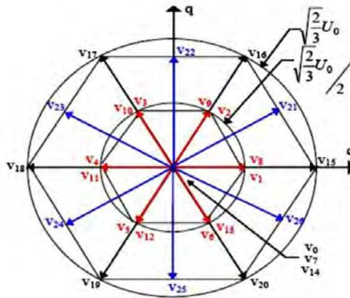
Fig. 2: Space vector diagram of three-level inverter
