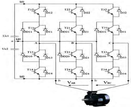
Fig. 1: Schematic diagram of a three-level inverter
