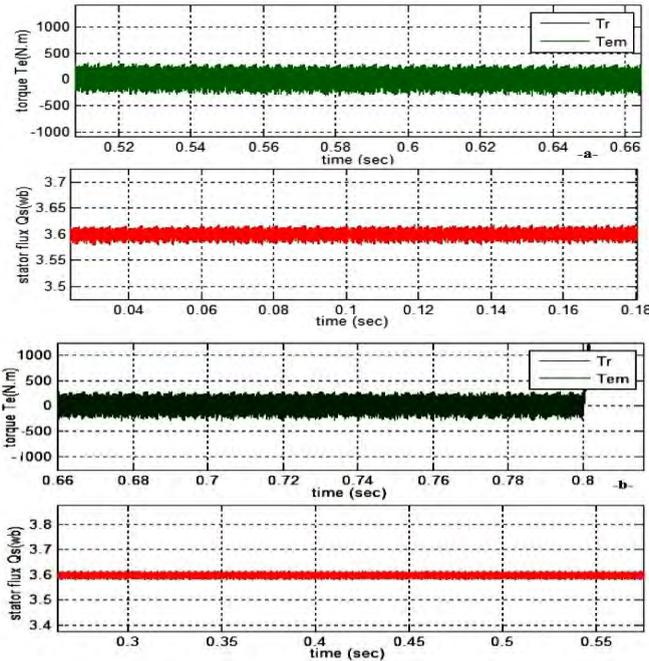
Fig. 13: Zooms of torque and flux: **a)** three-level DTC with 24 sectors, **b)** three-level DTC with 24 sectors based on artificial intelligence techniques
