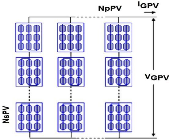
Fig. 1: Synoptic diagram of a PV generator
