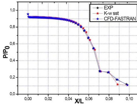
Fig. 5: Distribution of the parietal pressure of the upper walls NPR = 3.80 . Comparison of our results with Sellam [2]
