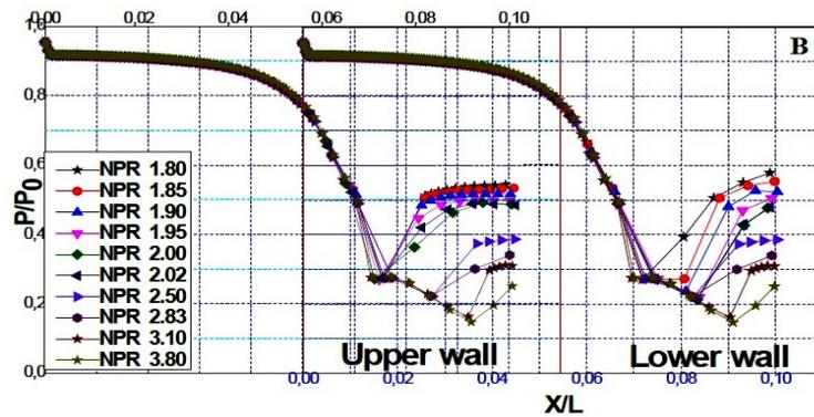
Fig. 8B: Comparison of pressure ratios (NPR decreasing)
