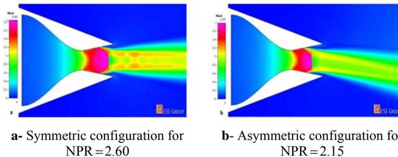
Fig. 6: Visualization numerical flow configuration at two different NPRs
