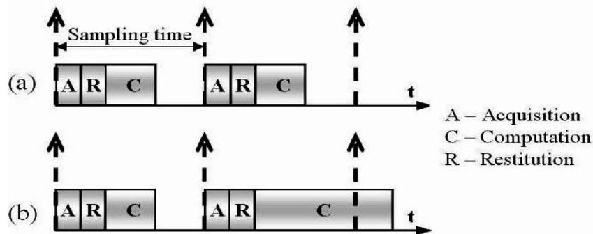
Fig. 5: RT simulator's tasks: (a) feasible and (b) unfeasible RT simulation
