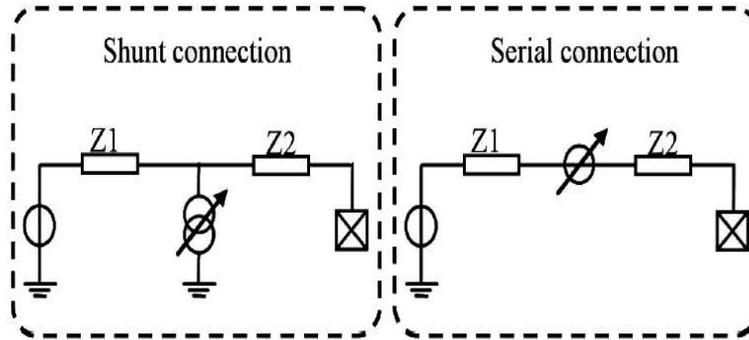
Fig. 2: Shunt and serial connections modelling
