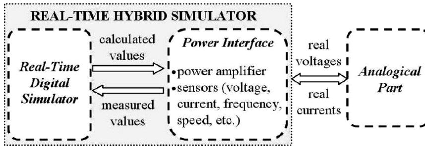
Fig. 8: Schematic diagram of a RT hybrid simulator
