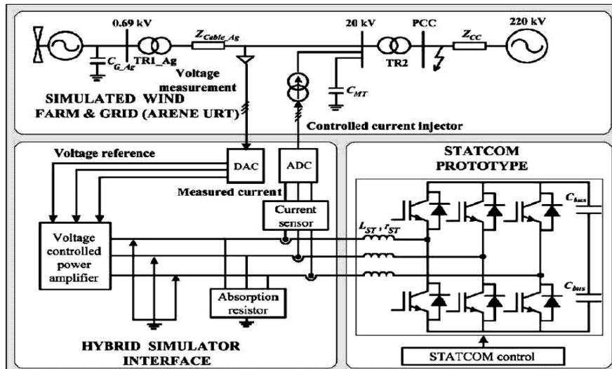
Fig. 11: RT PHIL simulation benchmark for D-STATCOM application
