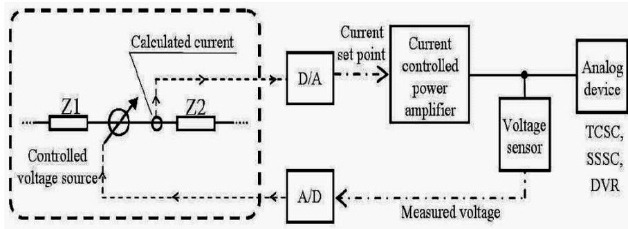
Fig. 4: Serial connection modelling for RT hybrid simulation
