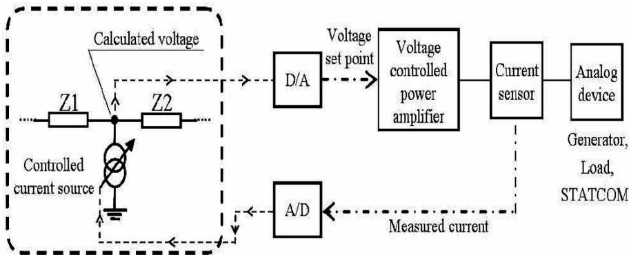
Fig. 3: Shunt connection modelling for RT hybrid simulation
