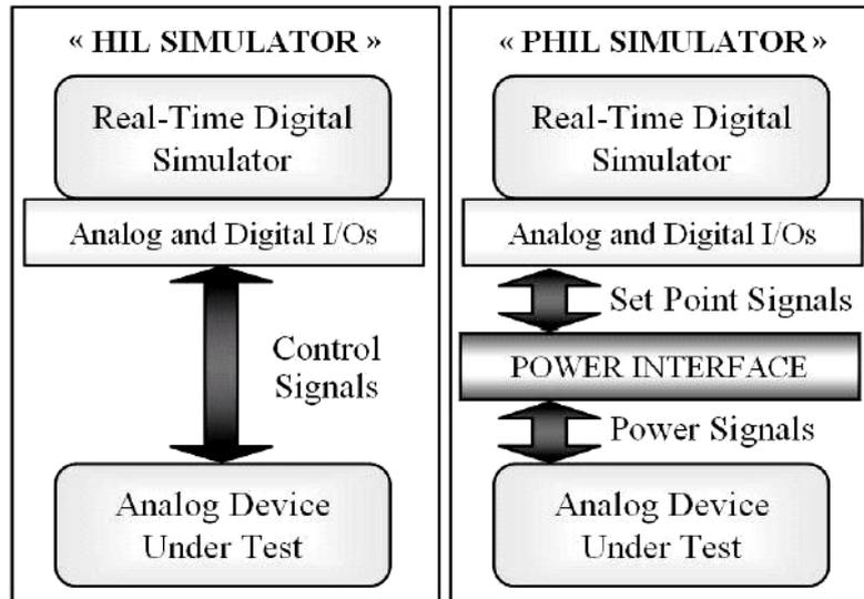
Fig. 1: Comparison between HIL and PHIL simulators
