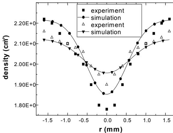
Fig. 3: Comparison of the radial neutral density profile from experiment and numerical model at two positions ( $z = 4.5$  mm and  $z = 2.5$  mm,  $z = 6$  mm represent the anode and  $z = 0$  mm represent the cathode)
