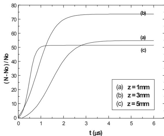
Fig.7: Temporal evolution of neutral density for three positions along the discharge axis - ( a ): near the cathode, ( b ): at the middle of the discharge, ( c ): near the anode
