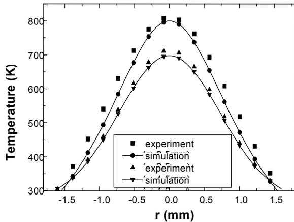
Fig. 4: Comparison of the radial neutral temperature profile from experiment and numerical model at two positions ( $z = 4.5$  mm and  $z = 2.5$  mm,  $z = 6$  mm represent the anode and  $z = 0$  mm represent the cathode)
