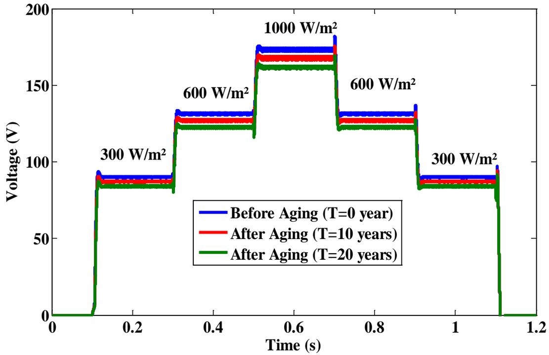
Fig. 23. PV Array voltage after 10 and 20 years
