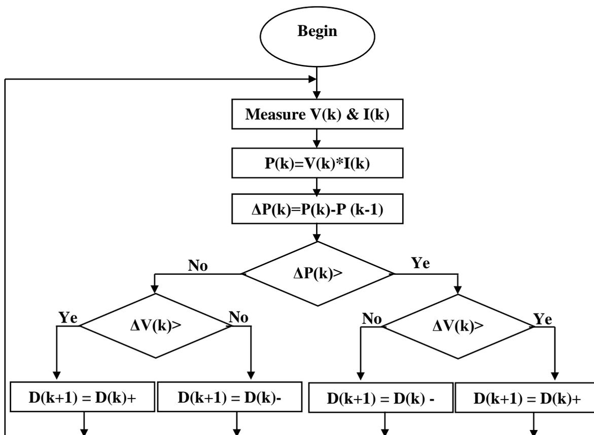
Fig.22. Flowchart of Perturb and observe algorithm [6];[22]
