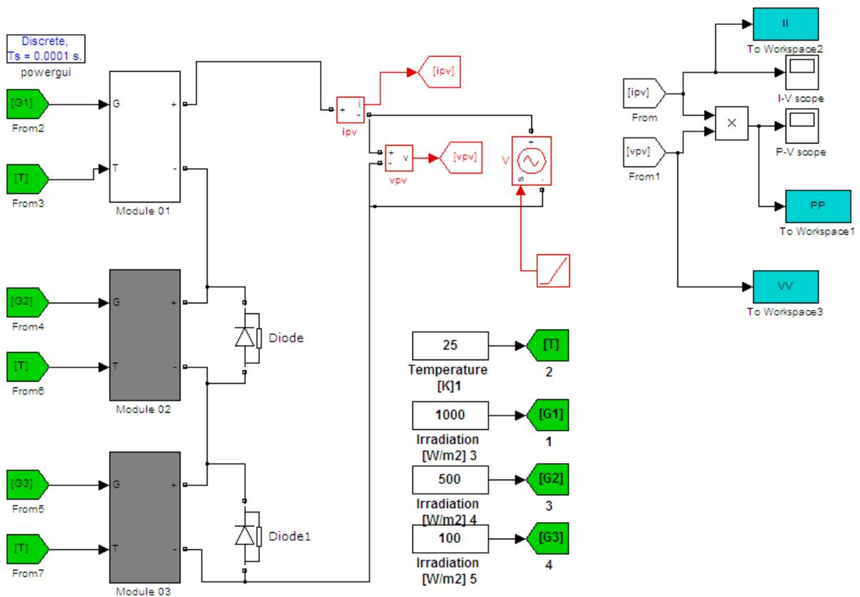
Fig. 16. Matlab/Simulink simulation of three series arrays.
