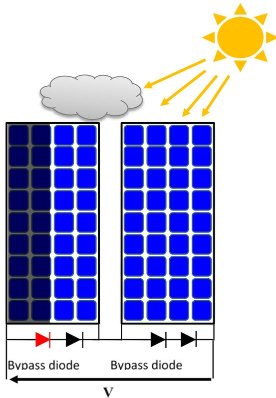
Fig. 13. Photovoltaic array under partial shading appearance
