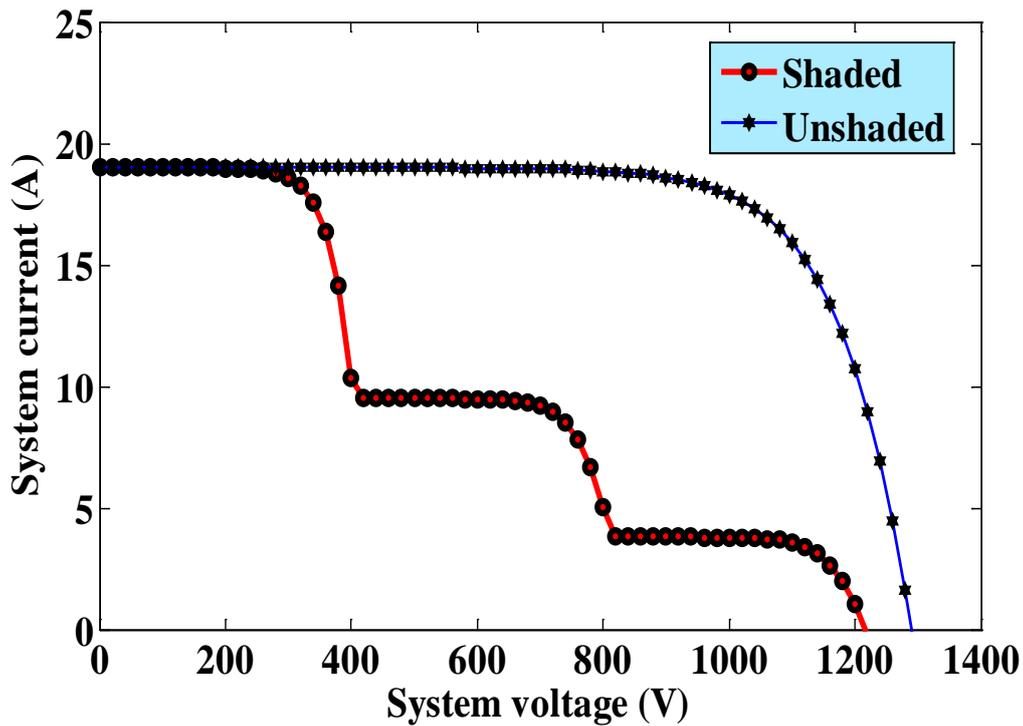
Fig. 17. I-V curves produced by three series-connected modules when two of them are shadowed (array 1  $G=1000\text{W}/\text{m}^2$ , array 2  $G=500\text{ W}/\text{m}^2$ , and array 2  $G=200\text{ W}/\text{m}^2$ )
