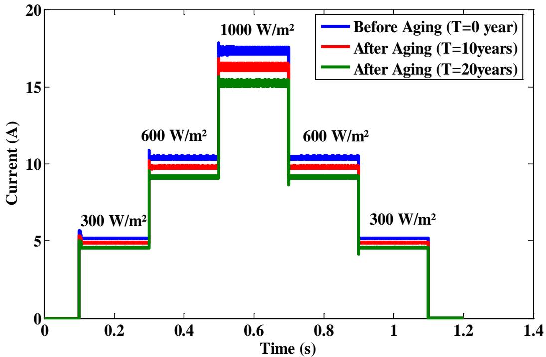
Fig. 24. PV Array current after 10 and 20 years
