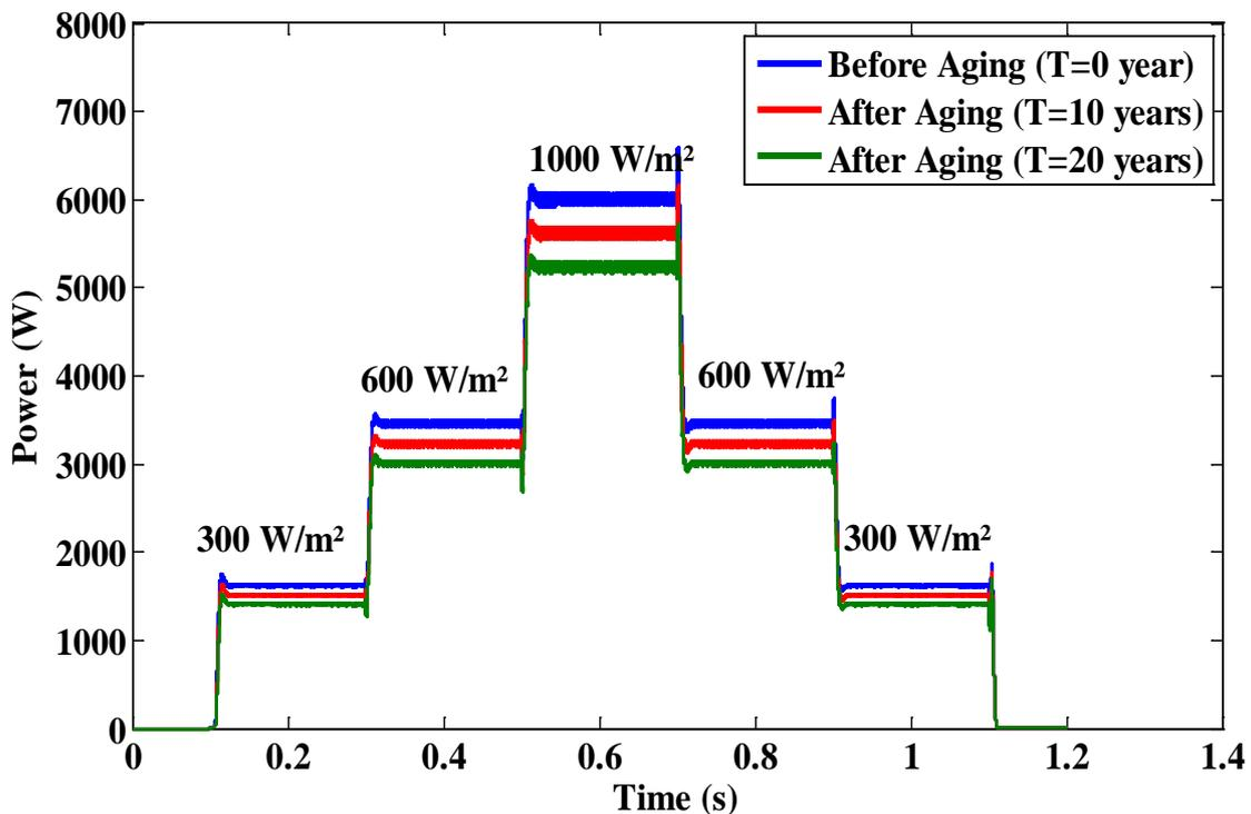
Fig. 25. DC-DC converter power after 10 and 20 years
