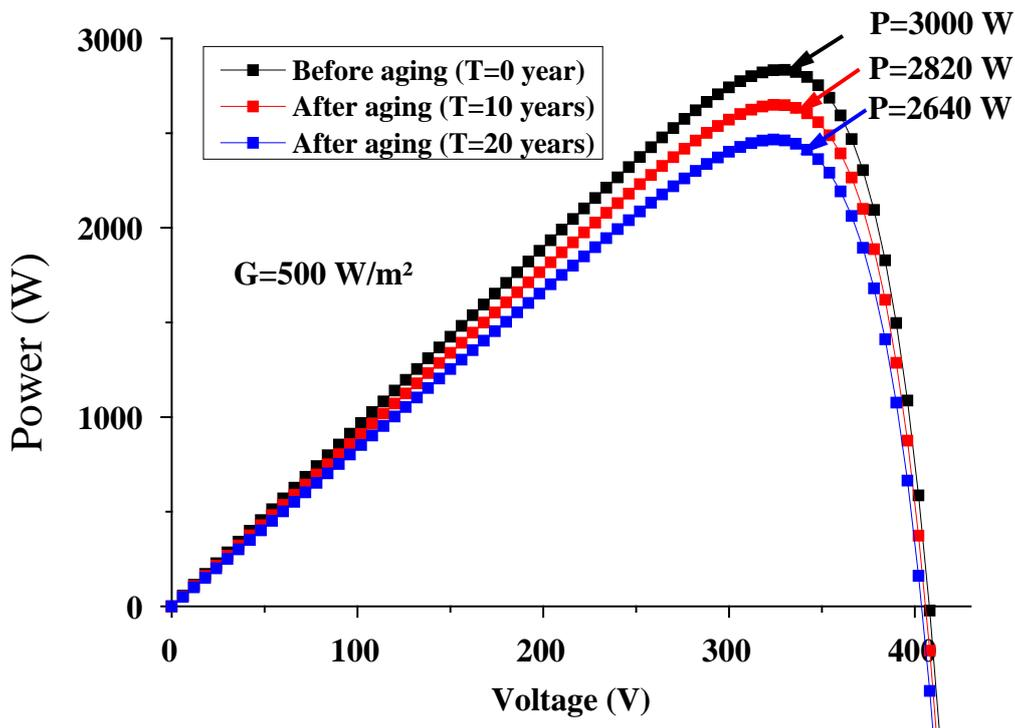
Fig. 19. Impact of aging on P-V characteristic of PV Array after 10 and 20 years for  $G=500 \text{ W/m}^2$
