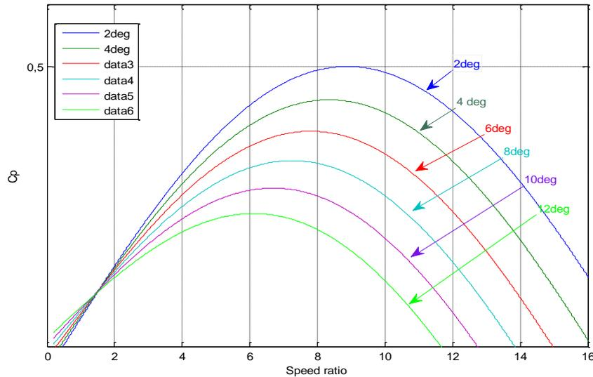
Fig.2 Characteristics of  $C_p(\lambda, \beta)$  for different values of  $\beta$
