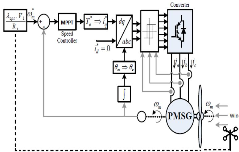
Fig1. Wind energy system using PMSG.
