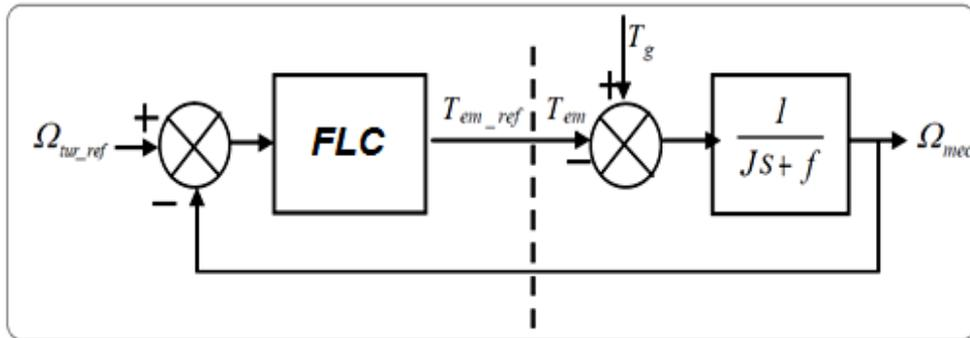
Fig.3 Diagram block of the FLC.
