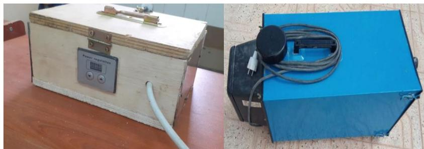
Fig. 4. Power regulation and aspirator respectively
