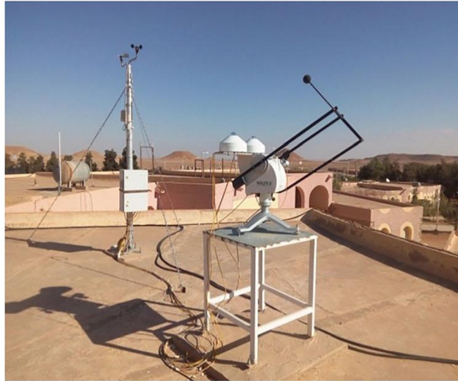
Fig 6. Instrumentations position for the measuring overall solar irradiance in per day.
