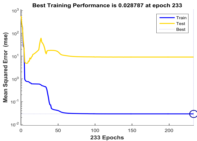
Fig 3. Training and Test results of heat transfer coefficient K_h based on the 6-3-1 configuration
