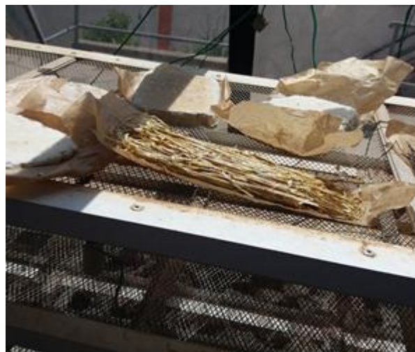
Fig 2. Milled straw block sample drying with natural convection in a solar greenhouse
