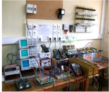
Fig. 2: Measuring equipments set up to characterize the photovoltaic panels and systems
