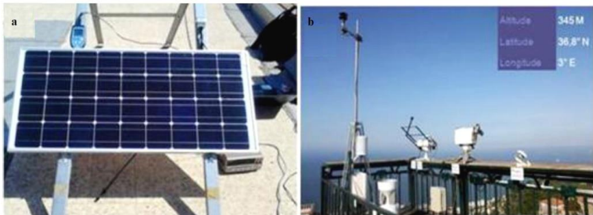
Fig. 2: -a- measurement of module PV temperature -b- metrological station of CDER
