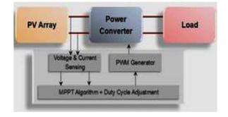
Fig. 2. PV system with MPPT controller
