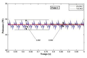
Fig. 10. **Point C**: Steady state oscillation i, case of fast changing atmospheric conditions.
