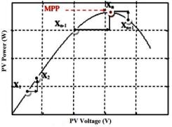
Fig. 3: P&O algorithm principle
