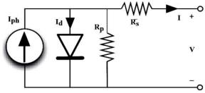
Fig. 1: Solar cell single-diode model
