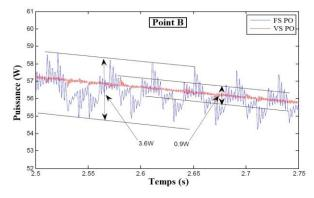
Fig. 9: Point B: Oscillation in case of soft changing atmospheric conditions
