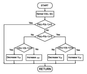
Fig. 4: Fixed step size P&O algorithm flowchart
