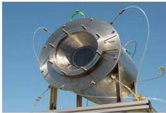
Fig. 1: Front view of the solar water-splitting receiver-reactor [1]
